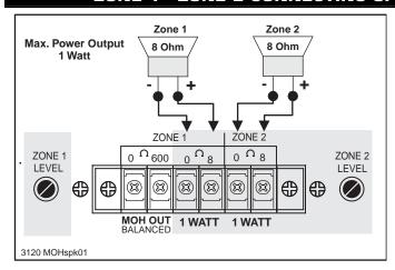
Fig 27 - Using one 8 ohm Speaker
